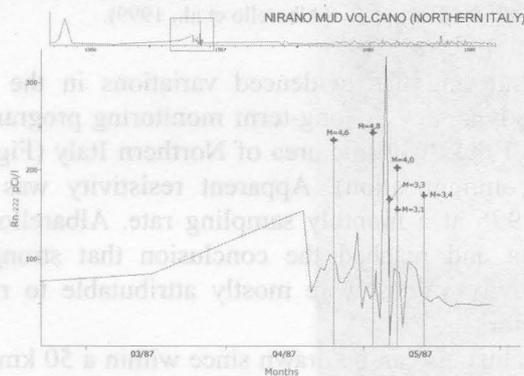
Figure 11. Radon fluctuations observed in Nirano mud volcano (North Italy) in 1986 – 1987 and local seismic events. After Martinelli and Ferrari (1991), modified.
