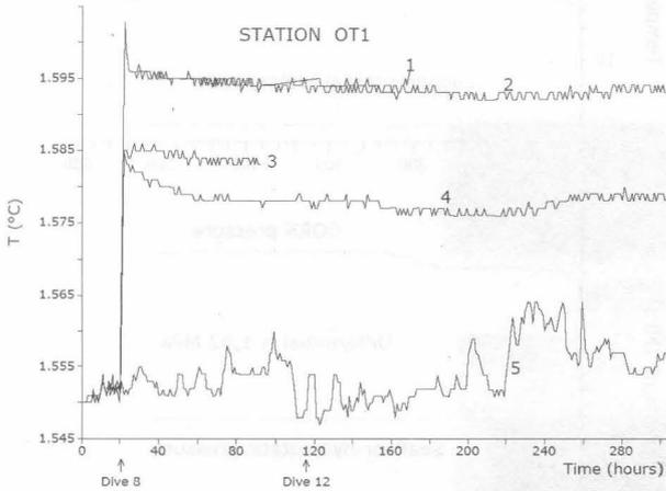
Figure 5. Graph shows temperature data collected at the Nankai accretionary complex. Record 1, 2, 3, 4 were collected at 64 cm depth (1 and 2), 44 cm depth (3) and 34 cm depth (4). Probe 5 was in sea water (Foucher et al., 1992).
