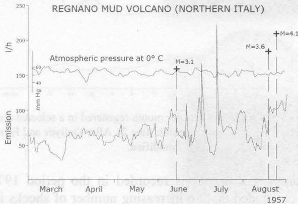
Figure 3. Methane flow-rate, atmospheric pressure and local seismic events recorded at the Regnano mud volcano, North Italy (Caneva, 1958; Martinelli and Ferrari, 1991).
