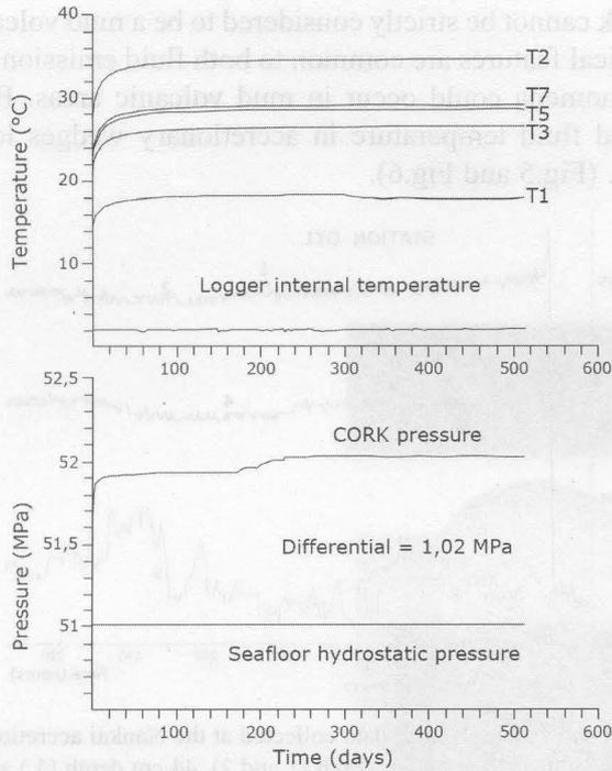
Figure 7. Long term records of temperatures and pressures measured in hole 949 C in Barbados accretionary prism (Becker et al., 1997)
