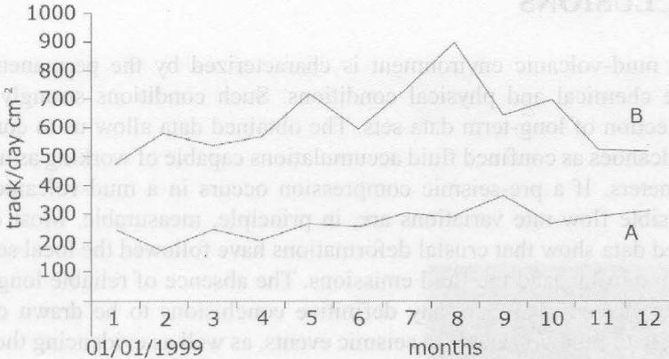
Figure 16. Radon fluctuations in the gas phase recorded in a mud volcano of the Taman area (Russia) in 1999 (Nevinsky et al., 2001).
